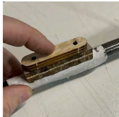
Once dry, lightly sand the mount with sandpaper on the boom
