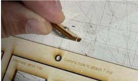
5. The T nut passes through the former
