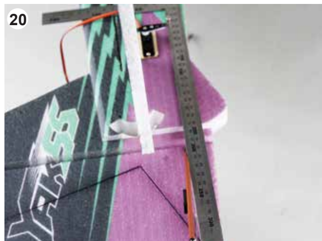
Use the same technique as shown above to prepare the control horn installation on the rudder.
