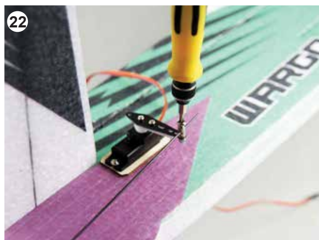
Install "Z-bend" pushrod as shown and lock it with the pushrod connector.
