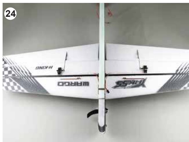
Insert carbon wing spar to one of the wing panel. Then insert it to the wing mount on the fuselage and put the other wing panel on and make sure it is well balanced and true to the fuselage.
