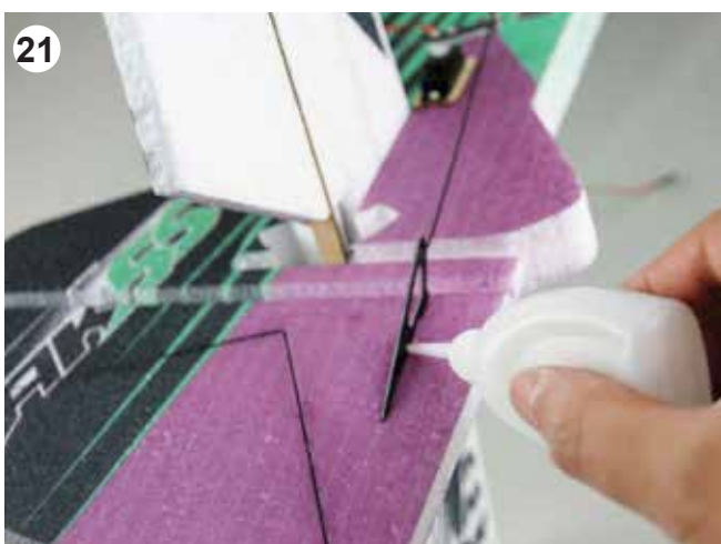
Apply CA glue to the rudder horn.
